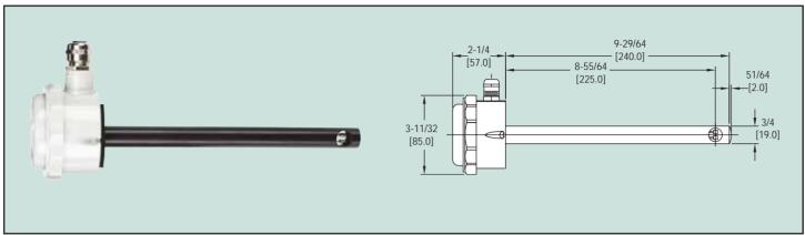
The Series AVU Air Velocity Transmitter is ideal for a wide range of HVAC measurement and control applications, particularly in complete building control and energy management systems. The Series AVU offers 5% accuracy at a surprisingly low cost, with six units covering ranges from 0-785 fpm to 0-3150 fpm, with either 4-20 mA or 0-10 VDC output.
